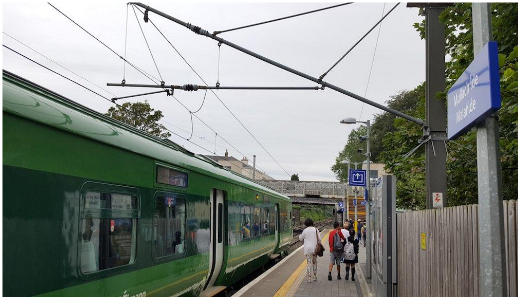
Figure 6-4: Existing single-track cantilevers at Malahide Station
